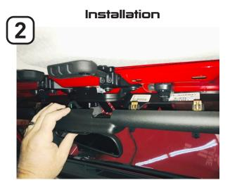
Start by pulling down firmly on the front of the factory header shroud to expose the wiring and connector for the warning lamp.
