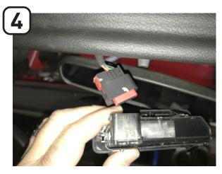
Press on the top of the red tab (closest to the wires) to release connector to the warning lamp.
