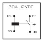
Please note: to operate properly, the ONE needs to switch the positive circuit, not the negative.
