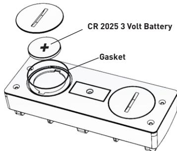
The Cr2025 Batteries should last several years, the reason for two is so that they will last a longer period of time, not for higher voltage.
