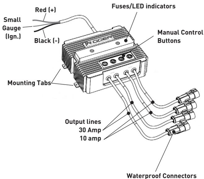
**CAUTION:** Do not exceed the recommended amperage limits shown here, may cause damage to the control module.
